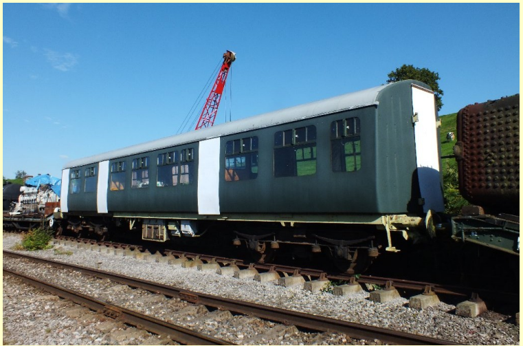
New protective door covers fitted to M59137 at Cheddleton, Churnet Valley Railway 29/9/13
